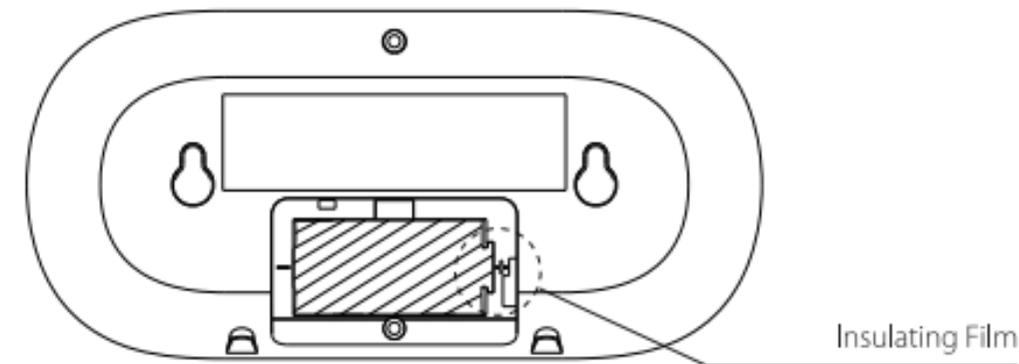
Before use, pull out the battery insulating film from the battery compartment to power on the device. After the device is turned on, the buzzer will beep once, the LCD backlight will light up, and the LED indicator will flash through 8 cycles (yellow/green/red). The device will then enter standby mode.
