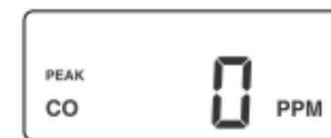
**Peak CO Concentration Reset:** During the 5 seconds when the LCD displays the peak CO concentration, press and hold the test button for 3 seconds, the device will beep, the LED will flash green, and the peak CO concentration will be reset with LCD displaying "0."
