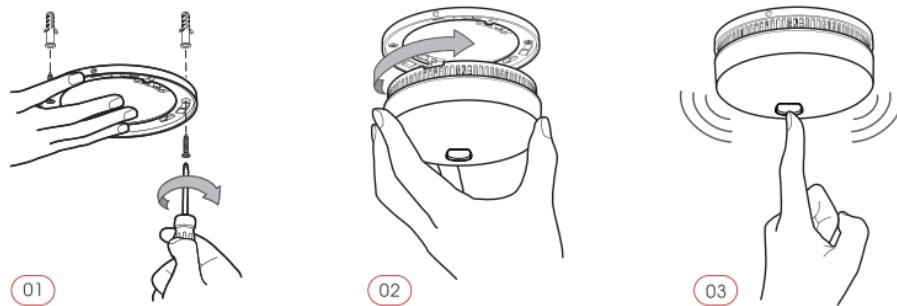
**NOTE:** If the mounting bracket is not attached to the alarm, be sure to hold down the activation button on the back of the alarm to turn it on while testing and connecting. Otherwise, it will not turn on.
